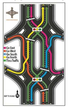
A Diverging Diamond Interchange, or DDI, temporarily channels traffic lanes to the left side of the roadway in order to create direct access with the interstate. The first one in Idaho is located at the interchange of I-86 and Yellowstone Avenue (U.S. 91) in Chubbuck. The diverging diamond interchange is a significant improvement in safety, since no left turns must clear opposing traffic and all movements are discrete, with most controlled by traffic signals.
