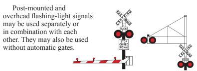
This active railroad control system has overhead and post-mounted flashing lights and an automatic gate.
